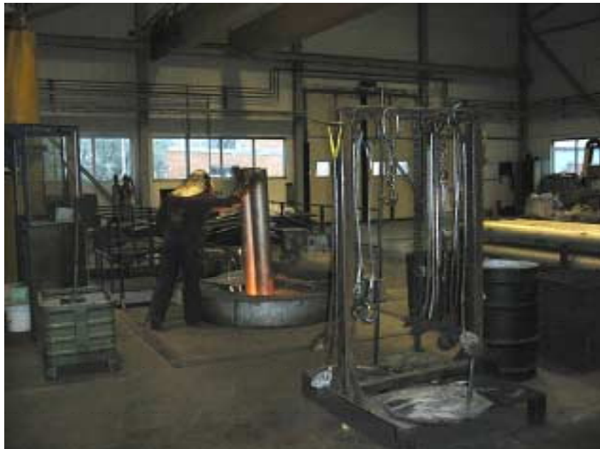
4. Feeding rack segment into melter.
